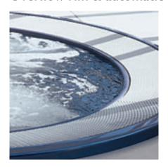
A distinctive feature of the Professional range and Profile Pro is the 15° angled overflow gird around the surface of the hot tub. It collects surface water, which overflows through the grid to a compensation tank. The water is then moved through a filtration system, cleaned and pumped back into the base of the hot tub to be re-used. Thanks to the slant of the grid the water remains at spa deck level even if there is a rocking motion, so they can be installed on yachts and ships.
