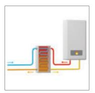
The Lodge range can be fitted with an upgraded electric heater or a heat exchanger, which is an inexpensive, green solution that exploits the heat produced by your facility's heating system or by renewable sources. To shorten heating time even further you can use the heat plus option in
